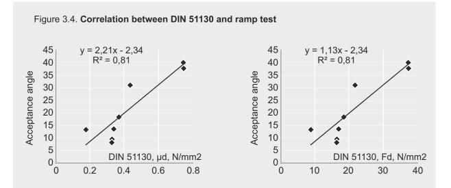
Latvijas Finieris does not publish any general uncommented sliding friction coefficients. The sliding friction coefficient of a friction-increasing surface depends on the combination of materials involved, the temperature, the condition of the material surfaces and the anti-slip mat (soiling, moisture, etc.). The contact surfaces of load and floor must be swept clean, grease-free and dry to achieve optimum anti-slip properties.
